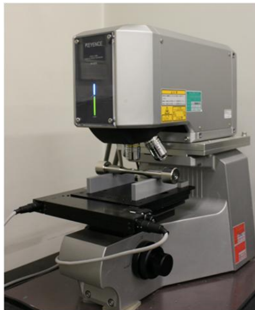
Fig. 2-9 Laser microscope (KEYENCE, VK-9510).
