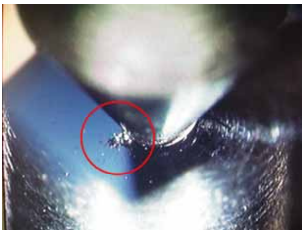
Fig. 6 (a) Schematic view of contact state between needle and specimen. (b): Photograph of hole-needle contact region. (Previous method)
